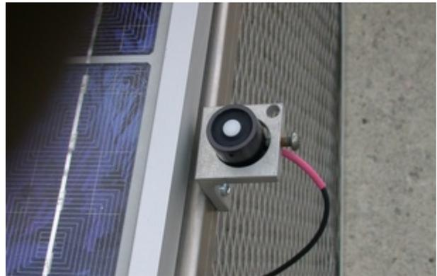
Fig. 2: Pyranometer mounting location.
